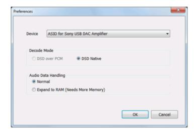
3. Select the device that you connected to the computer from the [Device] drop-down list, and then click [OK].
