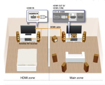
There are restrictions on the audio sources that can be used in Zone 2/3 or the HDMI zone. For details, see "Available inputs for each zone."
