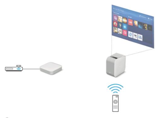
Connect the IR Blaster to the IR BLASTER connector of the Wireless unit.
