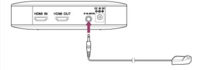
Mount the IR BLASTER head on the HDMI device so that the head is aimed at the remote control receiver of the device.
