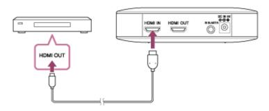
To also display images from the HDMI device onto a TV screen, connect the Wireless unit's HDMI OUT connector and the TV's HDMI IN connector with an HDMI cable (sold separately).
