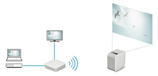
Connect the Wireless unit's HDMI IN connector and the HDMI device's HDMI OUT connector with an HDMI cable (sold separately).
