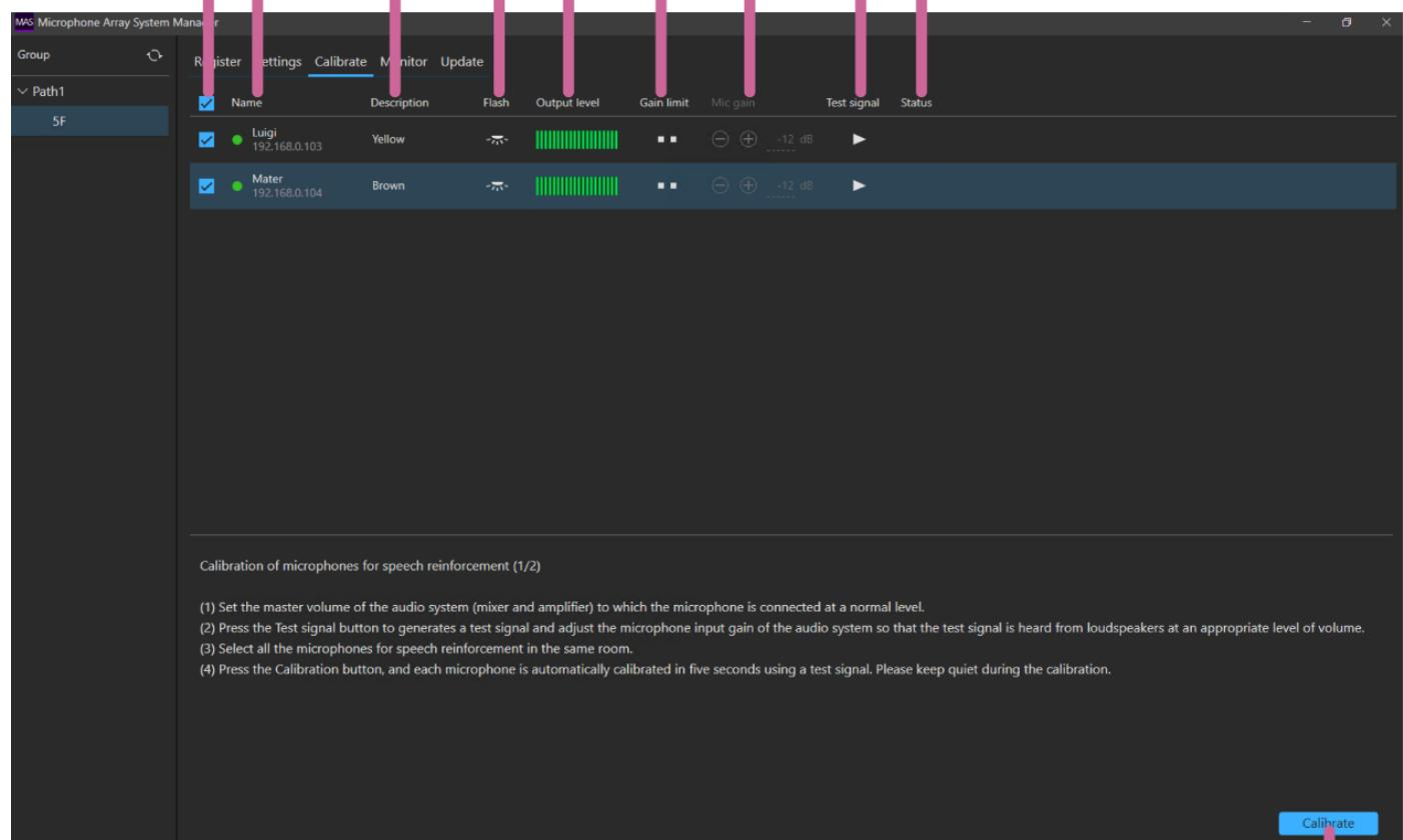
Calibration of microphones for speech reinforcement (1/2)
