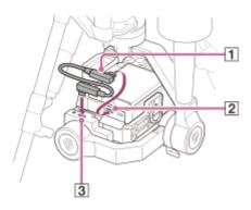
Make sure that the USB Type-C® cable (gimbal — camera) is properly connected.
