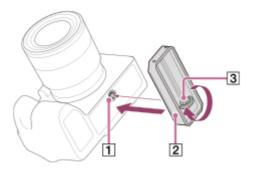
Attach the hot shoe adapter (4) to the camera.
