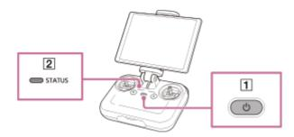
1 Press and hold the  $\circlearrowleft$  (Power) button (1) on the remote controller for at least 2 seconds.
