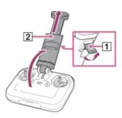
Place the mobile device on the mobile device holder and adjust the holder height.
