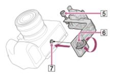
Pass the camera fixing screw (5) through the hook for the shoulder strap (8) on the camera and secure it.
