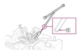
**4.** Turn the landing gear levers (2) until they are positioned in place. When storing the aircraft in the outer box, turn both landing gear levers (2) below the dotted line as shown below.
