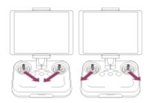
2. Operate the control sticks on the remote controller to make the aircraft ascend.
