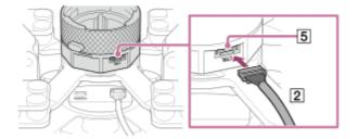
Connect the control cable (aircraft — gimbal) (2) to the control port (5).
