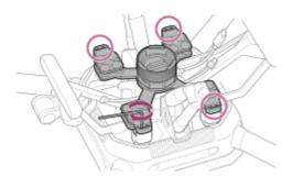
Insert the plugs at the other ends of the cables connected to the aircraft in the corresponding quick-release ports.
