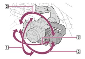
Adjust the balance of the tilt axis.
