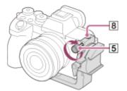
5 Adjust the mounting angle so that the L-Bracket (2) and the camera are oriented parallel.
