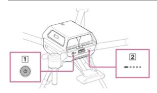
1 Press and hold the 🖰 (Power) button (1) on the aircraft for at least 2 seconds.
