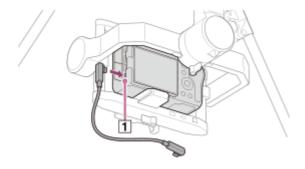
Insert the other end of the USB cable connected to the camera in the gimbal USB port ([2]).
