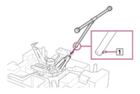
Make sure that the ball detent (1) is fully engaged.
