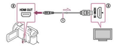
1. Switch the setting of this product according to the resolution of the connected 4K or high definition TV.
