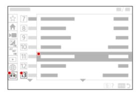
If newer camera software is available, a red notification badge will appear over the (Setup) tab, [Setup Option], and [Version] in the menu screen to notify you that an update is available (when the camera's system software (firmware) is Ver.2.00 or later).
