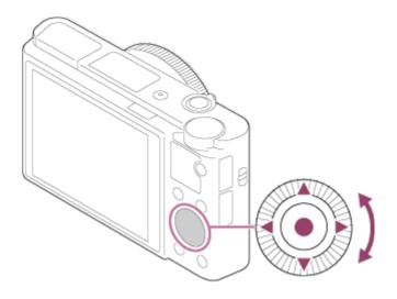
You can select setting items by turning or pressing the top/bottom/right/left side of the control wheel. Your selection is determined when you press on the center of the control wheel.
