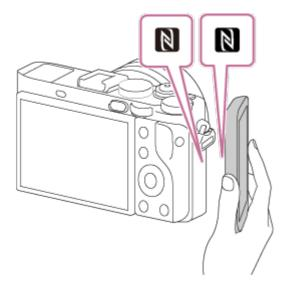
The product and the smartphone are connected, and PlayMemories Mobile automatically launches on the smartphone, and then the displayed image is sent to the smartphone.
