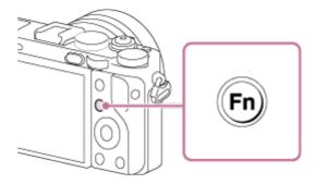
2. Select a function to be registered by pressing the up/down/left/right side of the control wheel.
