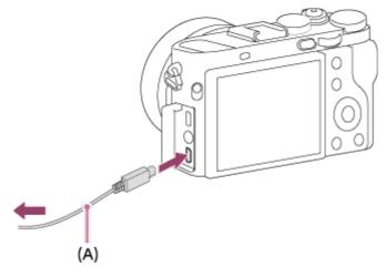
• If you connect the product to your computer using the micro USB cable when [USB Power Supply] is set to [On], power is supplied from your computer. (Default setting: [On])
