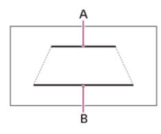
**A.** 2.0 m (6 1/2 feet) behind the car **B.** 0.5 m (1 3/4 feet) behind the car
