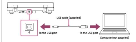
Use the USB cable supplied with the turntable to connect the computer and the turntable.
