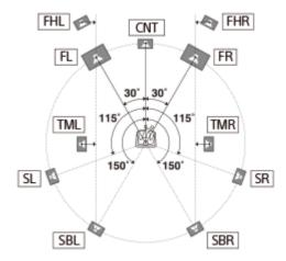
• **Type B:** Places four surround speakers at virtually identical angles, according to Recommendation ITU-R for 7.1 channel speaker placement.
