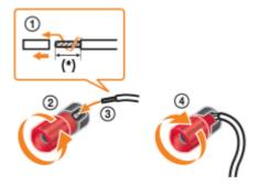
\* Strip the jacket to 10 mm (13/32 in) at each end of the speaker cables.
