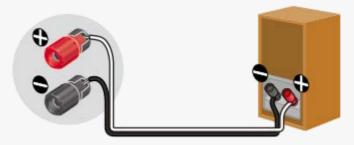
Improper connection may result in fatal damage to the receiver.
