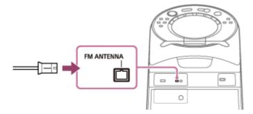
Extend the antenna (aerial) horizontally. Keep the antenna (aerial) away from the AC power cord (mains lead) and the USB cable to avoid picking up noise.
