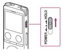
While the IC recorder is turned on, sliding the POWER • HOLD switch to [HOLD] displays [HOLD] and the current time for about 3 seconds on the display window, indicating that all the buttons on the IC recorder are disabled.
