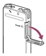
[2] Insert the microSD card into the microSD card slot until it clicks into place, and then close the slot cover.
