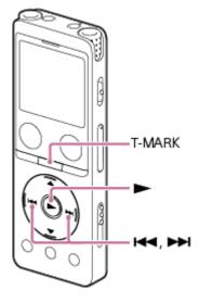
While recording is in progress or paused, or while playback is in progress or on standby, press T-MARK at the point you want to add a track mark.
