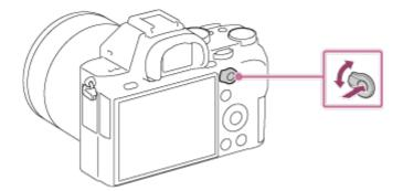
The exposure is locked, and \* (AE lock) lights up.
