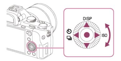
You can select setting items by turning or pressing the top/bottom/right/left side of the control wheel. Your selection is determined when you press on the center of the control wheel.
