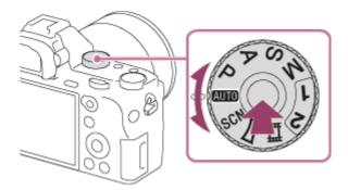
Turn the mode dial while pressing the mode dial lock release button in the center of the mode dial.
