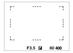
• When you use a zoom function other than the optical zoom, the [Focus Area] setting is disabled and the focus area frame is shown by the dotted line. The AF operates with
