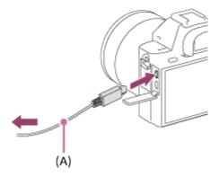
If you connect the product to your computer using the micro USB cable when [USB Power Supply] is set to [On], power is supplied from your computer. (Default setting: [On])
