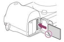
• With the notched corner facing in the direction illustrated, insert the memory card until it clicks into place. Insert the memory card correctly. Not doing so may cause a malfunction.
