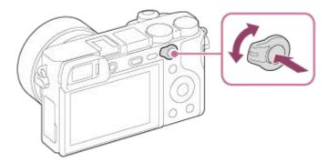
The exposure is locked, and \* (AE lock) is displayed.
