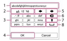
Move the cursor on desired key using the control wheel, then press the center to enter.
