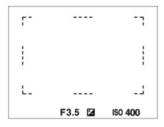
When you use a zoom function other than the optical zoom, the [Focus Area] setting is disabled and the focus area frame is shown by the dotted line. The AF operates with priority on and around the center area.
