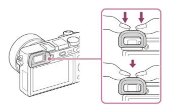
To remove the eyepiece cup, grasp it on the left and right sides and lift it up.
