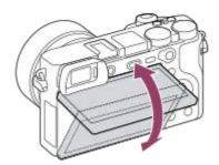
You may not be able to adjust the monitor angle depending on the type of a tripod you use. In such a case, release the tripod screw once to adjust the monitor angle.
