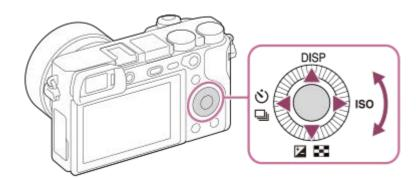
• You can select setting items by turning or pressing the top/bottom/left/right side of the control wheel. Your selection is determined when you press the center of the control wheel.
