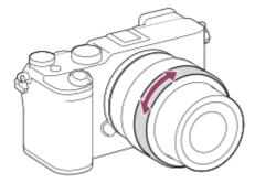
• When you shoot a still image, you can display the focus distance on the screen by rotating the focusing ring. The focus distance is not displayed when the Mount Adaptor (sold separately) is attached.
