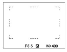
• When you use a zoom function other than the optical zoom, the [Focus Area] setting is disabled and the focusing frame is shown by the dotted line. The AF operates with priority on and around the center area.
