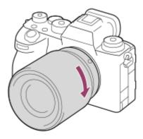
Be sure to hold the lens straight when attaching it.
