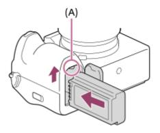
3 Close the cover and slide the switch to the LOCK side.
