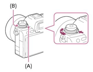
Turn the focus mode dial **(B)** while holding down the focus mode dial lock release button **(A)** to select the desired mode.
