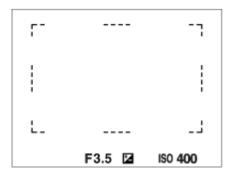
• When you use a zoom function other than the optical zoom, the [ Focus Area] setting is disabled and the focusing frame is shown by the dotted line. The AF operates with priority on and around the center area.
