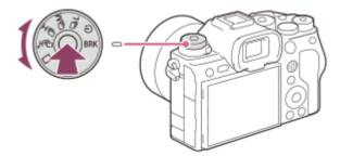
Turn the drive mode dial while holding down the drive mode dial lock release button in the center to select the desired mode.
