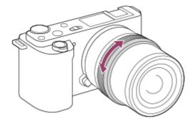
• When you shoot a still image, you can display the focus distance on the screen by rotating the focusing ring. The focus distance is not displayed when the Mount Adaptor (sold separately) is attached.
