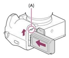
Close the cover and slide the switch to the LOCK side.
