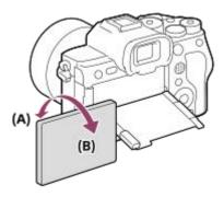
In the default settings, the inversion of the display is automatically switched on and off depending on how the monitor is positioned. You can lock the display method with the following settings: MENU → (Setup) → [Finder/Monitor] → [Monitor Flip Direction].
