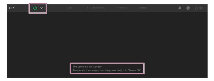
In this state, press the power switch and select [Power ON] from the switch menu. The unit turns on, the POWER lamp lights up green on the front of the unit, and the camera image appears on the live operation screen of the Web App.
