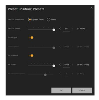
Select [Pan-Tilt Speed Unit] > [Time] and set the transition times (Pan-Tilt/Zoom) you want to change using the sliders or enter values directly and press the [OK] button.
