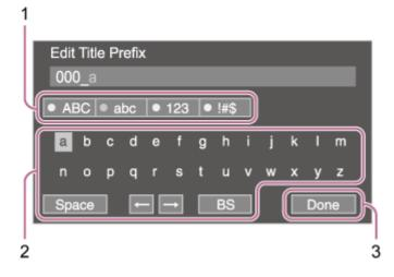
Press the arrow buttons in the GUI control panel to select the character type and apply the setting.
