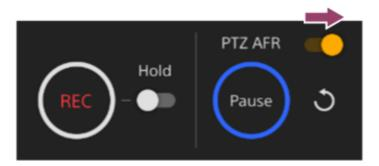
The camera image automatically moves to the start position. Auto tracking starts when a person enters the detection area.
