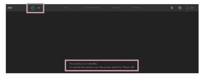
To turn the power on again, press the power switch and select [Power ON] in the switch menu.
