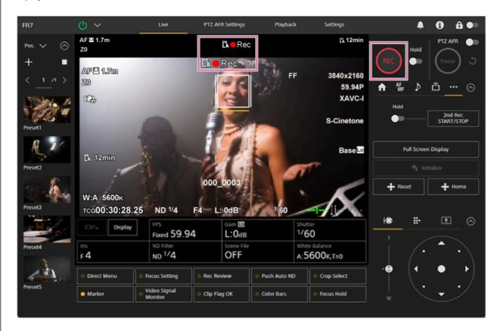
5 To stop recording, press the record START/STOP button again.
