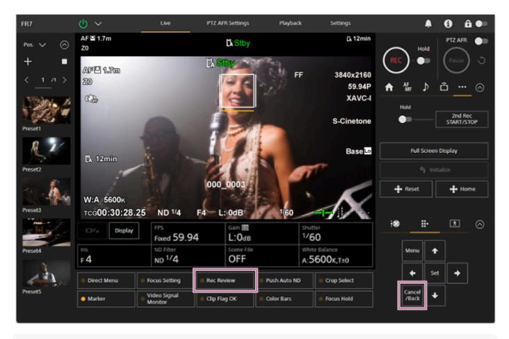
You can also press the [Cancel/Back] button of the supplied infrared remote control to stop the Rec Review function.
