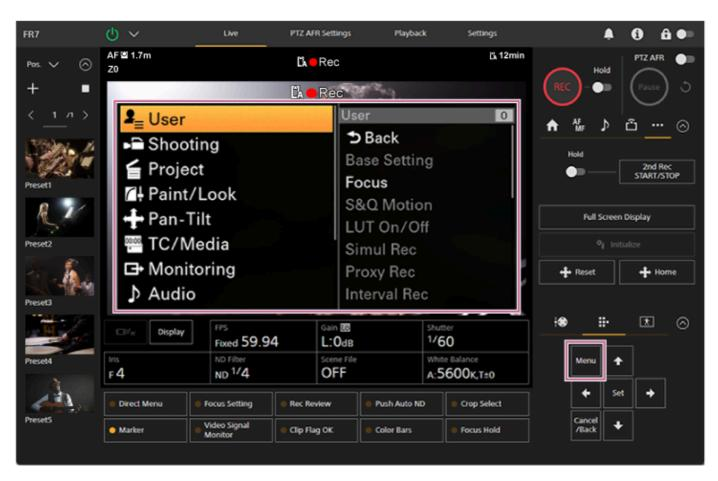
You can configure the settings required for shooting and playback using the camera menu. Press the [Menu] button while the camera menu is displayed to hide the camera menu. The camera menu is operated using the GUI control panel.
