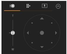
When pan/tilt operation is not initialized or needs to be reset, you can quickly access the (Pan/tilt reset) button in the camera control panel by pressing the message displayed below the joystick.
