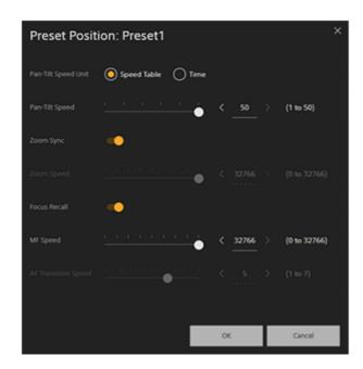
Select [Pan-Tilt Speed Unit] > [Speed Table] and set the transition speeds (Pan-Tilt/Zoom/Focus) you want to change using the sliders or enter values directly and press the [OK] button.
