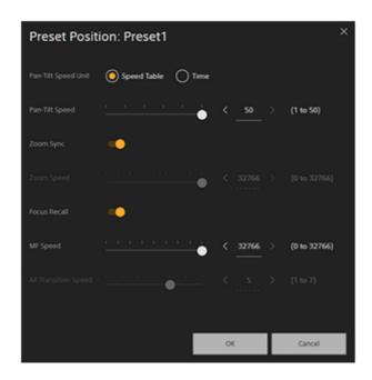
Slide the [Zoom Sync] switch to the right to turn the function on and press the [OK] button.
