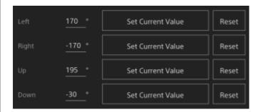
The limit positions are set and are displayed as numeric values (angle). To cancel a limit, press the [Reset] button for the individual positions.
