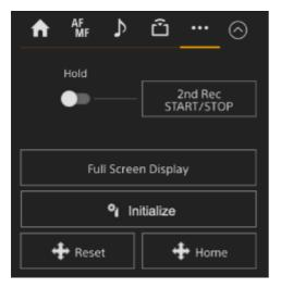
Pressing the [Full Screen Display] button opens a new tab in the web browser and displays the camera image panel image in full screen.
