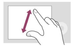
During single-image playback, you can enlarge or reduce the displayed image by moving apart or bringing together two fingers on the screen (pinch-out/pinch-in).
