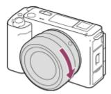
Be sure to hold the lens straight when attaching it.
