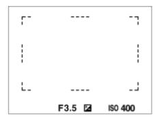
• When you use a zoom function other than the optical zoom in the still image shooting mode, the [ } Focus Area] setting is disabled and the focusing frame is shown by the dotted line. The AF operates with priority on and around the center area.
