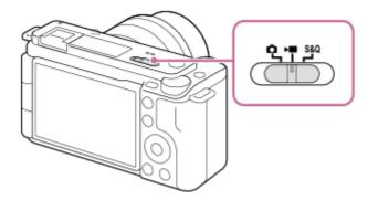
You can select the still image shooting mode, movie recording mode, or slow-motion/quick-motion recording mode as the shooting mode using the Still/Movie/S&Q switch.
