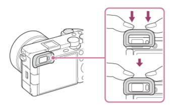
To remove the eyepiece cup, grasp it on the left and right sides and lift it up.
