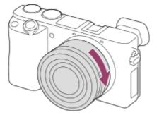
• Be sure to hold the lens straight when attaching it.
