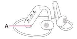
A: Microphone on the remote control component
