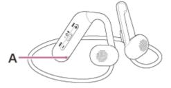
A: Microphone on the remote control component
