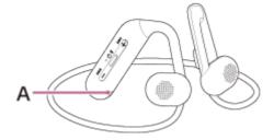
A: Microphone on the remote control component
