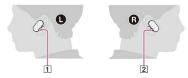
While both units of the player are on your ears, hold down the button (1) for 2 seconds to turn on the Bluetooth function.
