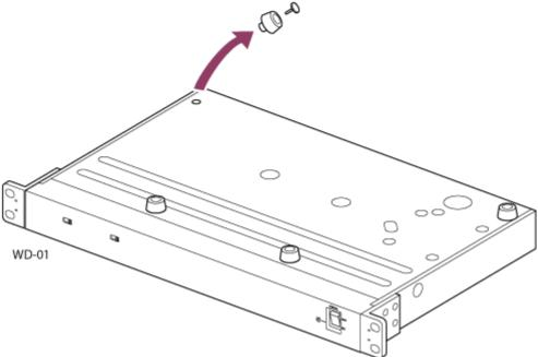
2 Attach the unit to the rack using screws (effective length 10 mm or longer) that match the screw diameter of the rack.
