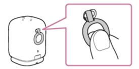
2. Twist the ring strap counterclockwise so that its attachment loop ( ① ) slips over the strap peg and shifts to the lower left of the peg.
