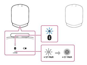
On the other speaker, press and hold the (BLUETOOTH)/ — ST PAIR (Stereo Pair) button for about 2 seconds.
