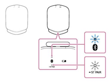
4 Check the state of the indicator on each of the 2 speakers.
