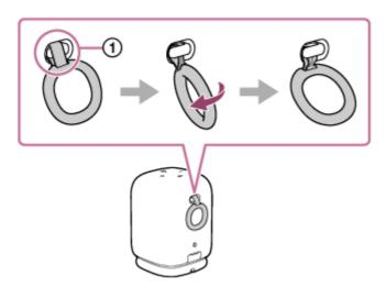
3. Pull the ring strap rightward with force to make its attachment loop shift underneath the strap peg and come off.
