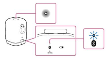
When the speaker has no pairing information, for example when you use the BLUETOOTH function for the first time after purchase, the (BLUETOOTH) indicator keeps double flashing in blue.
