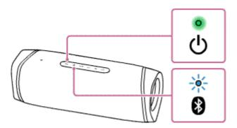
When the speaker has no pairing information, for example when you use the BLUETOOTH function for the first time after purchase, the \( \mathbb{R} \) (BLUETOOTH) indicator keeps double flashing in blue.
