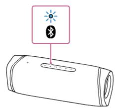
After you pair the speaker with a BLUETOOTH device for the first time since purchase or initialize the speaker (the speaker has no pairing information), the speaker automatically enters pairing mode when it is turned on. Proceed to step 4.
