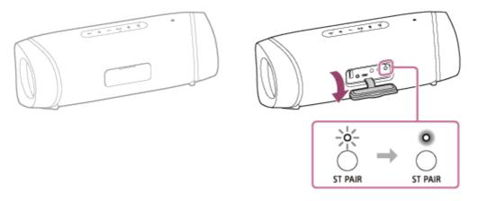
When a connection for the Stereo Pair function is established, the ST PAIR (Stereo Pair) indicators on both speakers stay lit and the (BLUETOOTH) indicator on either of the speakers turns off.
