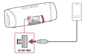
When you connect the speaker to an AC outlet, the connected USB device starts to be charged automatically. If the speaker is being powered by the built-in battery only, proceed to step 2.
