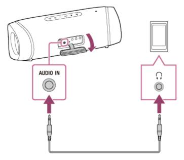
1 If you use an audio cable (with stereo mini plugs) with significant resistance, the sound may be lower. Therefore, make sure you use a cable (with stereo mini plugs) without resistance.
