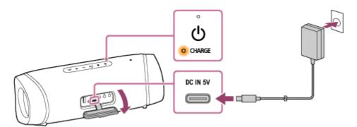
Battery charging starts and the CHARGE indicator lights up in orange. Charging will complete in about 5 hours and the indicator will turn off.
