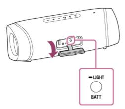
By pressing and holding the button for about 3 seconds again, the lighting function turns on/off again.
