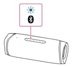
After you pair the speaker with a BLUETOOTH device for the first time since purchase or initialize the speaker (the speaker has no pairing information), the speaker automatically enters pairing mode when it is turned on. Proceed to step § .
