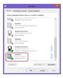
If you cannot click [Connect] for [SRS-XB43 Stereo], select [Disable] for the [Default Device] that currently has a checkmark (green).
