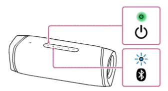
When the speaker has no pairing information, for example when you use the BLUETOOTH function for the first time after purchase, the (BLUETOOTH) indicator keeps double flashing in blue.
