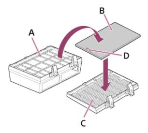
Pull the pull stick (D) upwards when removing the air filter from the dust cover assembly. When attaching the air filter to the air filter cover, make sure the correct side is being attached so that the pull stick is protruding from the air filter.
