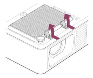
Remove the air filter from the air filter cover.
