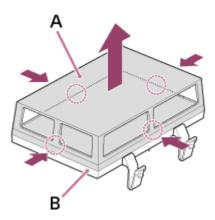
Remove the air filters (A) and (B) from the filter frame.
