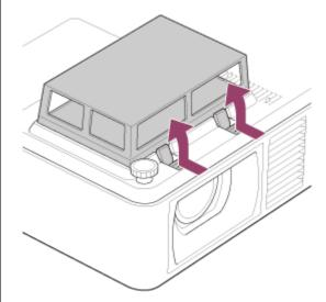
Push all four sides of the dust cover to loosen the hook, and then remove the dust cover (A) from the filter frame (B).
