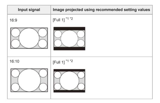
\*1 Selecting [Normal] will project the image with the image signal resolution as-is without enlargement processing.
