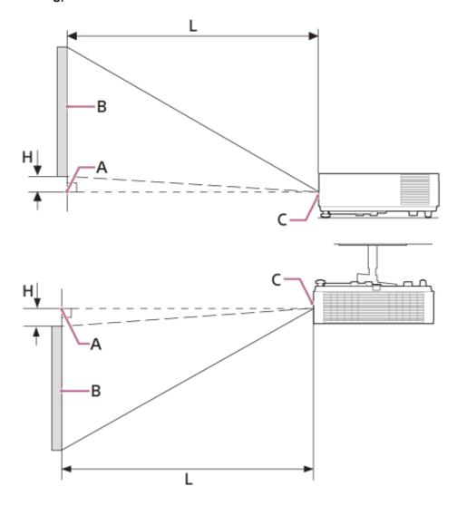
**A:** The point of intersection of the line drawn perpendicular to the surface projected from the lens center and the projection surface
