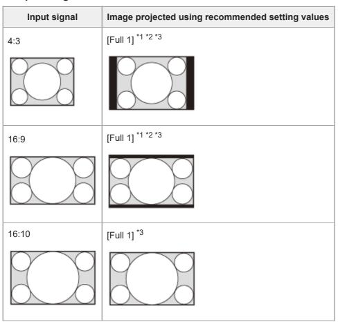
\*1 Selecting [Normal] will project the image with the image signal resolution as-is without enlargement processing.
