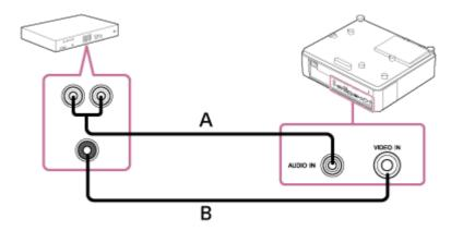
A: Audio cable (Pin plug x 2 - Stereo mini plug) (not supplied)
