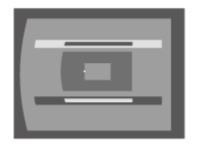
You can adjust the center point of deflection using the ♠/♣ (Up/Down) keys. For the range of deflection, use the ♠/♠ (Left/Right) keys. You can adjust the left/right side independently.
